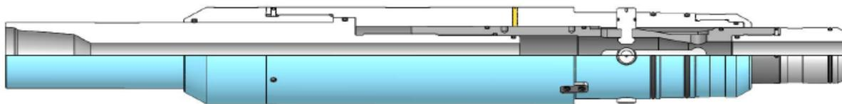
The Mechanical Obtain/Retrieval Tool (MOT) that is used to retrieve the Retrievable Bridge Plug (RBP) is slightly different than the MOT used for retrieving the Hydraulic Retrievable Hangers (HRH). When an HRH is set, the well has communication through the inside of the hanger. When an RBP is set, the well has no communication through the inside of the plug. This difference in tools require a different function when obtaining/retrieving them from the wellbore.
