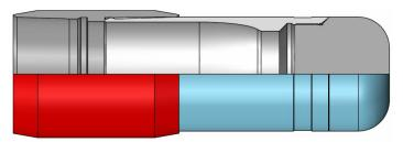
Bull Nose Shoe (BNS) is a tool that is installed on the bottom of a tubular string. The purpose is to close off the Casing or Tubing string from having access to the outer annular that it resides in. It will eliminate any multi-phase fluid and gas influxes into the casing string. The BNS allows the tubular string to contain pressure for injection and production purposes. The BNS also acts as a guide when running tubular strings into a well.
