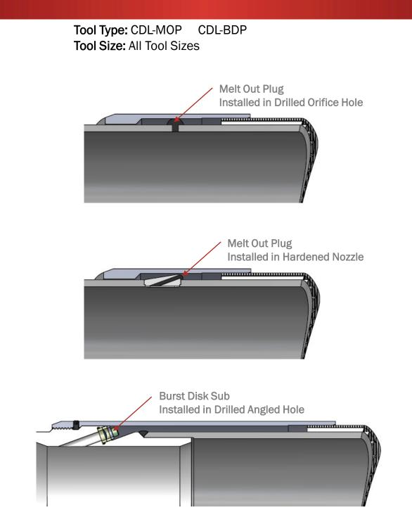
All tools are custom designed. Customer would receive technical data sheet with actual dimensions, threads and performance data.
